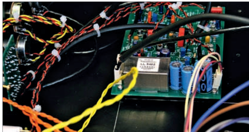
Glasgow EMP Lecturer Andy Jackson, showing his build of the 1176 Audio compressor. The unit was built for SAE Glasgow.
