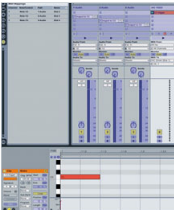
Picture 4, 5: Each note can be assigned to an audio or MIDI clip's play button. Single note can be also assigned to any amount of clips resulting in multiple clips playback.
